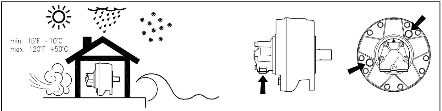
**Make sure that all the oil supply, discharge, drainage or other motor ports are closed.**
