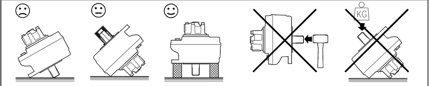
**Make sure that the shaft of the motor is not loaded in any way and is protected from knocks.**
