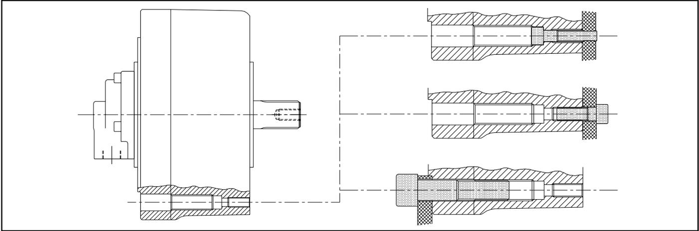
NOTE: Installation type 1.) P05 and GM05 Series, with thru bolt M10, use washer size 10.5x18x2.
